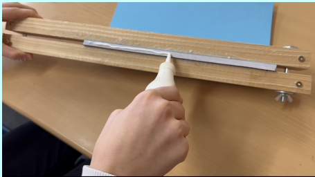
13. Put on wood glue twice (needs about 10 minutes to dry).
